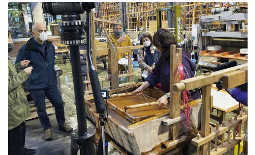
和紙会館での紙漉きを行う様子 Making paper by hand at Awagami Factory
